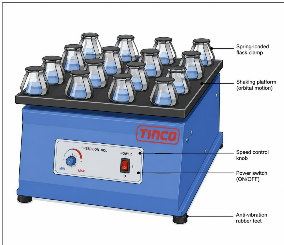
Figure 2: Schematic of an orbital flask shaker used for microbial culture and bioprocess incubation.
